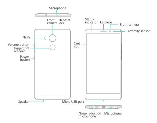
Do not cover the proximity sensor, as this will affect some of the phone's functions. If you use a screen protector, do not cover the sensor. Use a screen protector that is designed for your phone with a purpose-built hole for the sensor.
