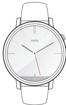
To **turn on**, press and hold the power button until your watch vibrates.
