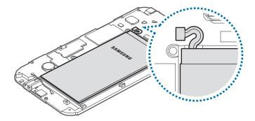
6 Push the back of the battery with your fingers and remove the battery.
