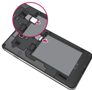
3. Insert the battery into place by aligning the gold contacts on the battery and the phone **1** and pressing it down until it clicks into place **2**.
