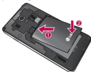
4. Align the back cover over the battery compartment and press it down until it clicks into place.
