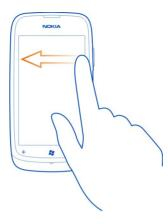
**Example:** Swipe left or right between the start screen and the apps menu, or between different views in the hubs. To quickly scroll through a long list or menu, slide your finger quickly in a flicking motion up or down the screen, then lift your finger. To stop the scrolling, tap the screen.
