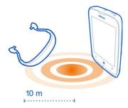
Paired devices can connect to your phone when Bluetooth is switched on. Other devices can detect your phone only if the Bluetooth settings view is open.
