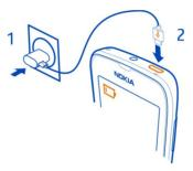
2 When the battery is full, disconnect the charger from the phone, and then from the wall outlet.
