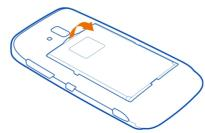
3 Make sure the contact area is facing down, and insert the card.
