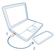
2 When the battery is full, first disconnect the USB cable from your phone, then from the computer.
