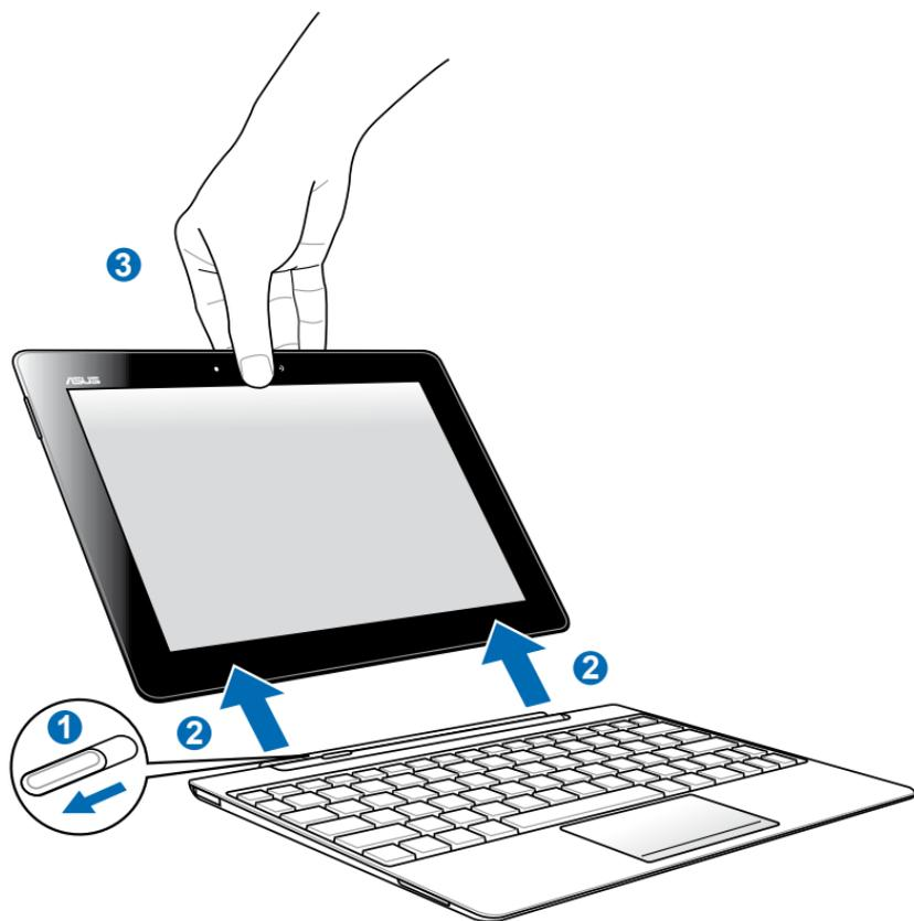
1. Use one hand to move the latch to the left to release the Eee Pad and stabilize the mobile docking.
