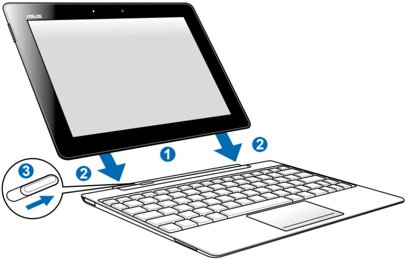
1. Align the Eee Pad with the mobile docking.
