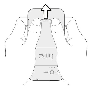
3. With your finger, lift up the back cover from the bottom side to remove it.
