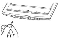
Press the RESET button with a small pin or clip. The screen will freeze; the Reader will not restart automatically.
