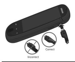
Note: This illustration displays both the correct and incorrect orientation for connecting the charger. If the charger is incorrectly connected, damage to the accessory port will occur, voiding the phone's warranty. 4. When charging is finished, first unplug the charger's power plug from the AC wall outlet, then disconnect the charger's connector from the phone.
