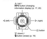
Operation guides displayed at the bottom of the screen indicate that the **MENU** button,  $\textcircled{\ \ }$  button, or zoom buttons can be used.
