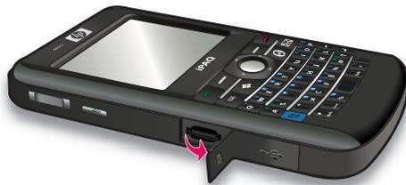
2. Slide the storage card in the MicroSD slot with the metal area inserted first and facing the rear of the HP iPAQ.
