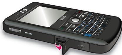
4. Push the card in the slot to unlock the card.
