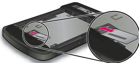
3. Slide the SIM card into the SIM card slot.
