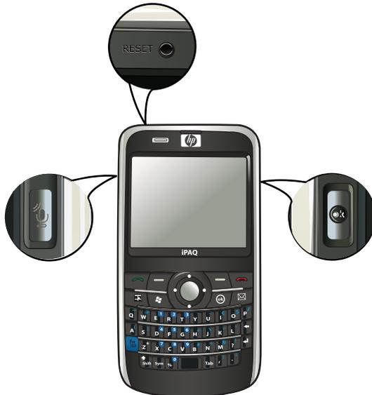
3. Keeping the **ok** and the **Voice Commander** buttons pressed, use the stylus to lightly press the **Reset** button.
