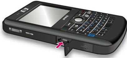
5. Remove the storage card from the storage card slot.
