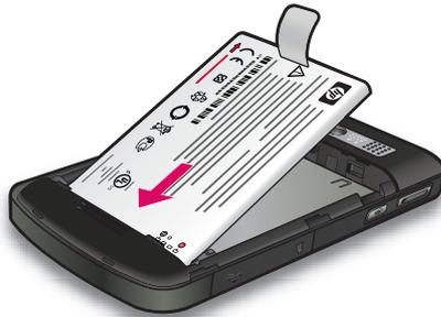
2. Place the battery cover down and slide up until it locks into place.
