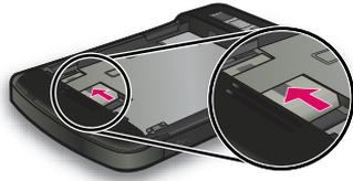
**NOTE:** If the battery is already installed, remove it before inserting the SIM card. The SIM card is provided by a mobile phone service provider. Also, make sure that the metal contacts are facing down and the notched corner is in the correct position. If the SIM card is not properly inserted in
