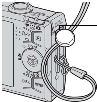
Hook your fingernail or the wrist strap toggle under the bottom edge of the A/V OUT and DIGITAL terminal cover to open it.
