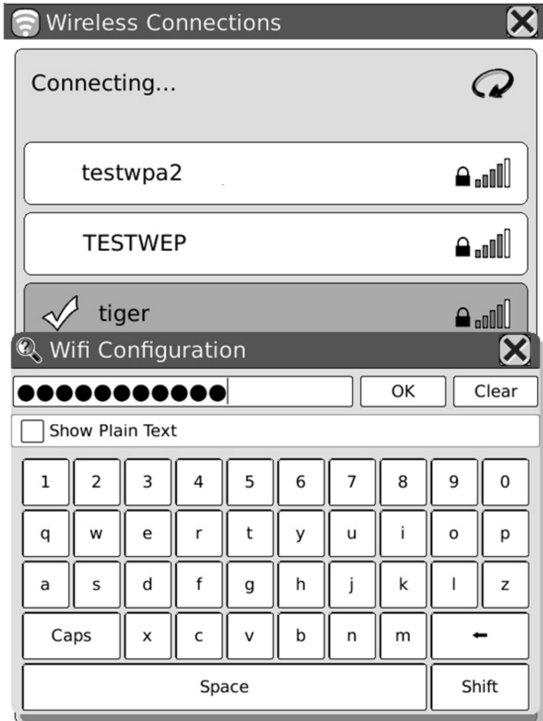
Fig. 7.12.4 Snapshot of Configuring WPA Security Access Point
