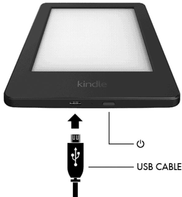
**Power button:** To turn your Kindle on, press the Power button. If you need to turn off your Kindle screen, press and hold the Power button for 7 seconds until the Power dialog displays, then select Screen Off.
